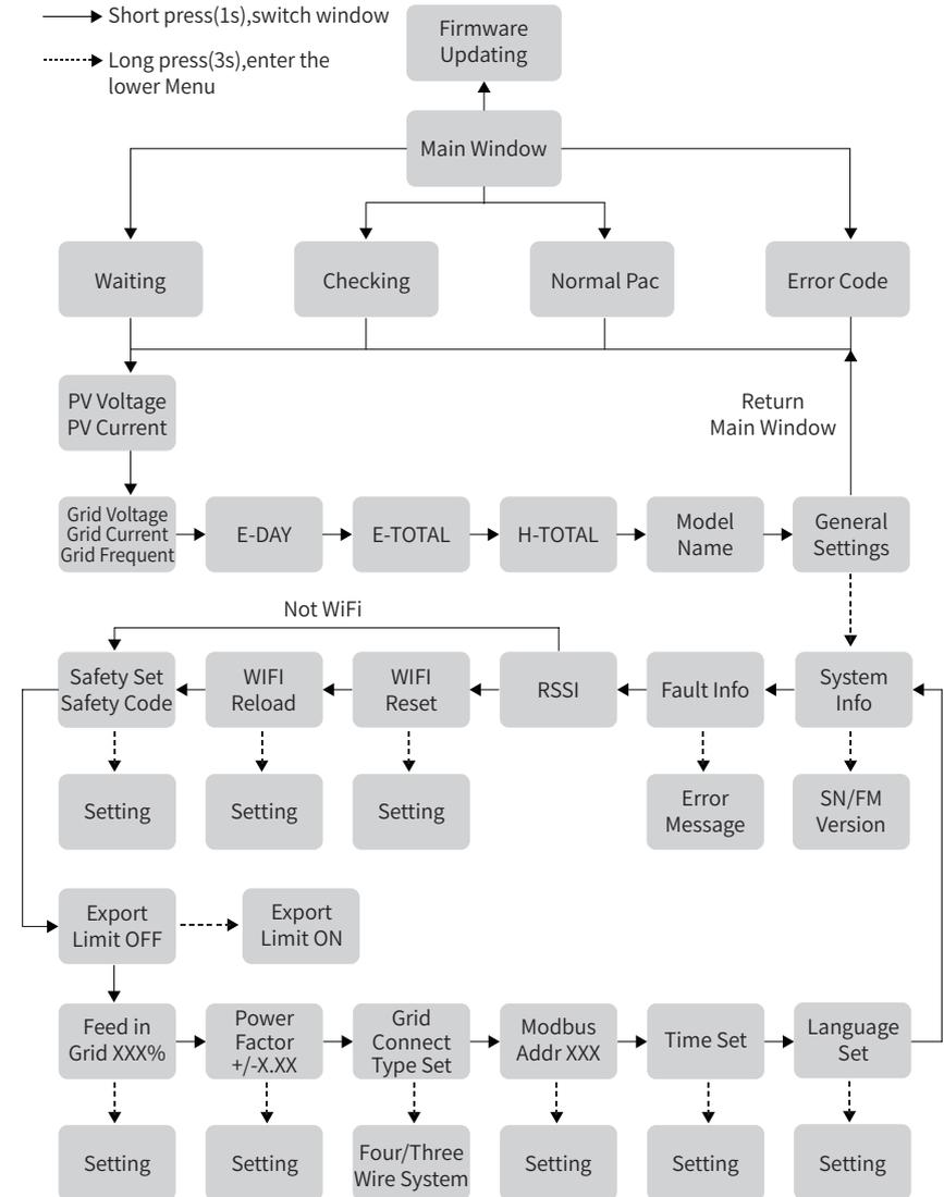
Tip: After every setting completed, wait for 10 seconds and the inverter will automatically save your settings or modifications.
