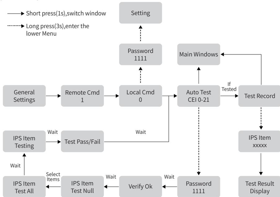
The auto test will start when the correct test item is selected, and the test result will be displayed on the screen when it finished. If the test success, it will display “Test Pass”, otherwise will display “Test Fail”. After each item tested, the inverter will reconnect to the grid and automatically start the next test item according to the requirements of CEI 0-21.
