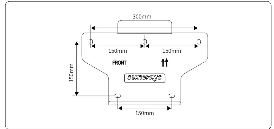
Figure 4-4 Dimensions of wall bracket
